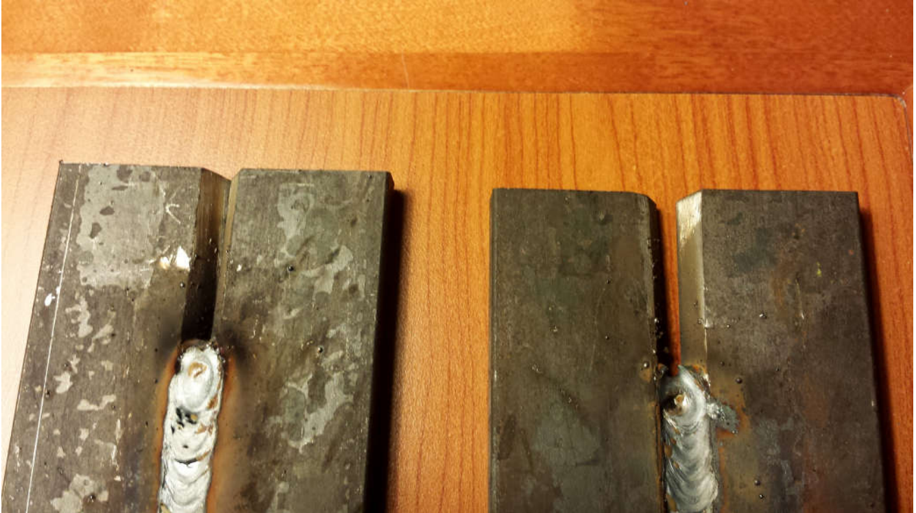
Vibrated sample on left, not-vibrated on right.
