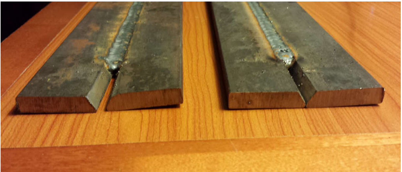
Not-vibrated test piece on left, vibrated on right.
